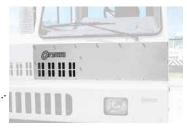
Large front access panel for easy access to front of engine, wipers, HVAC.
