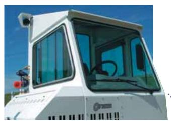
Large glass area and cab design provide excellent visibility to the front, rear and sides.
