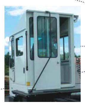
Large diameter, comfortable grab handles, easy-opening sliding rear door mean quick, comfortable entry, exit.
