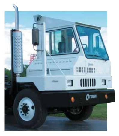
The air-ride cab is designed for quiet comfort, convenience and reduced maintenance. Large cab pivot bushings are designed to help lower cab noise levels and reduce wear to bushings and pins. Raised cab models have no top windows to create solar heating, glare. Electric tilt is standard equipment.
