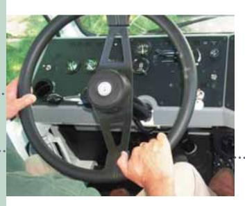
Instrument panel features low-glare, easy to clean ABS material. Heavy-duty gauges are circuit grounded for greater reliability. LED lighting and lighting displays provide long service life. Dash can be serviced without removing steering column.
