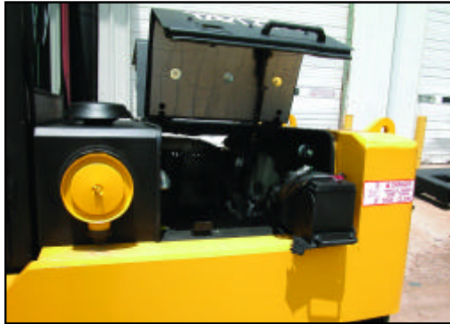
Gull wing hood allows for easy service access to engine compartment and slide-out battery.
