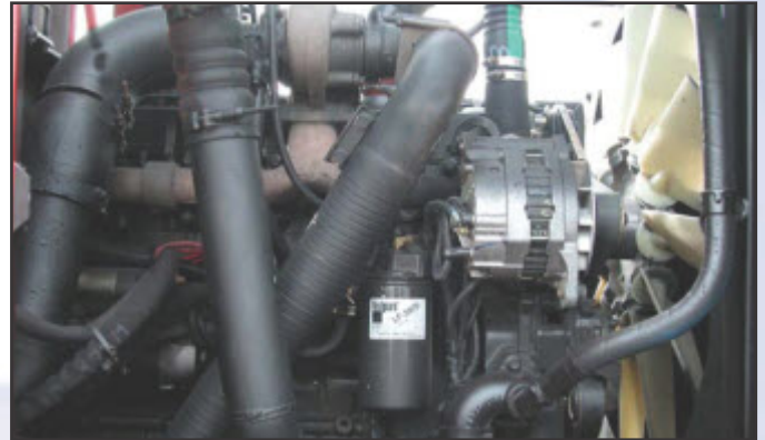
Cummins QSB5.9-C230, 6-cylinder turbocharged engine
