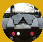
**Tapered rear frame** assists easy hook-up by raising trailer to fifth wheel height during engagement.
