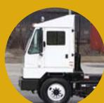
**Air-ride cab with large pivot bushings** provide a quieter, more comfortable ride and reduce wear to bushings and pins.
