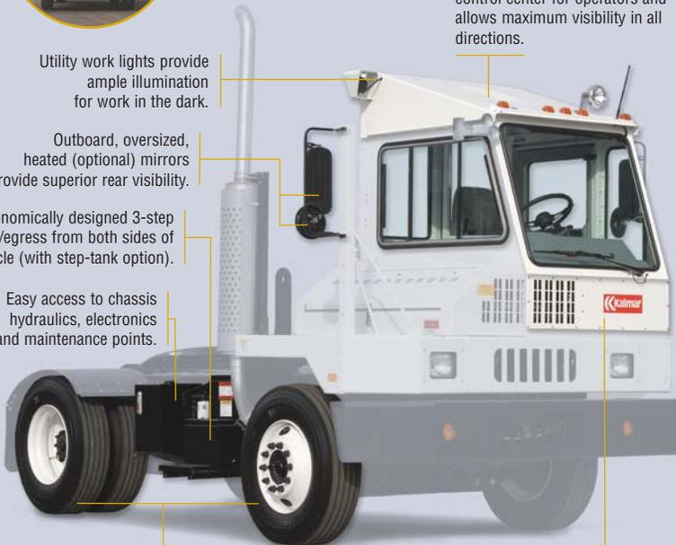
Short wheelbase, sharp turning radius, DOT approved mechanical linkage power steering for ease of operation and high maneuverability.
