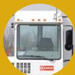
**Oversize windows and mirrors** are designed and placed to give drivers full visibility in all directions in all weather conditions.
