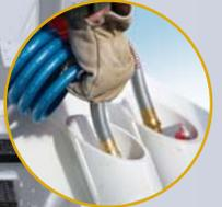
Full operator deck provides secure footing and maximum work access to air lines and trailer connections.
