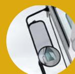
**Heated mirror options** provide improved visibility and less start-up time in cold, icy weather.
