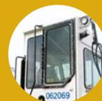
**Window guard options and cab protection options** are custom-fitted and provide increased safety for operators.
