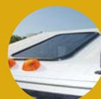
**Roof skylight option** provides additional visibility and light in working situations where overhead sight is important.
