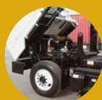
**Tilt cab and front access panel** provide full access to tractor drivetrain and components for repair or maintenance.
