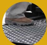
**Integrated cab floor, catwalk and rear deck** are constructed from self-cleaning steel tread and provide a stable work area.
