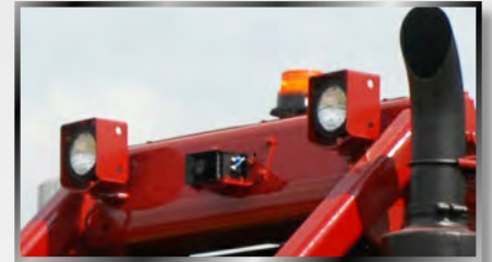
Overhead rear work lights for improved safety and visibility Key-switch actuated amber strobe light Reverse activated alarm
