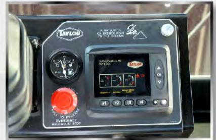
Easy to understand diagnostic display. TICS (Taylor Integrated Control System) using CANbus technology is standard on the TX Series.
