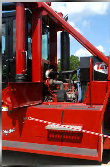
Battery cut-off switch
