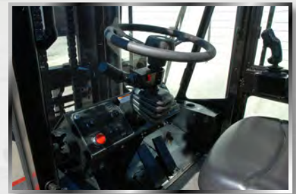
Spacious uncluttered cab with tilt steering, hinge-down dash, climate controls and adjustable seating Premium vinyl or cloth seat that rotates 15° left and 20° right
