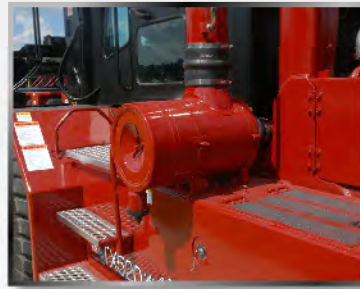
Dual element air cleaner with restriction indicator
