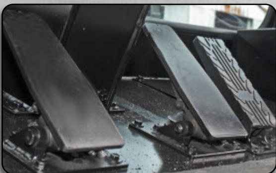
Two brake pedals left – brakes and inching right – brakes only
