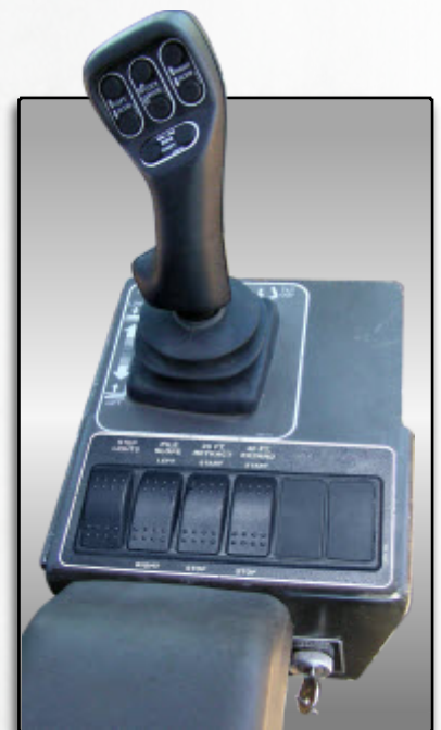
Joystick control with individual fingertip hydraulic and electronic controls for smooth precise control
