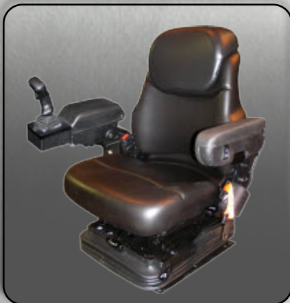
Premium vinyl or cloth adjustable air suspension seat with arm rests, orange seat belt, and OPS (operator presence switches) (Rotation 15° - left - 20° - right)
