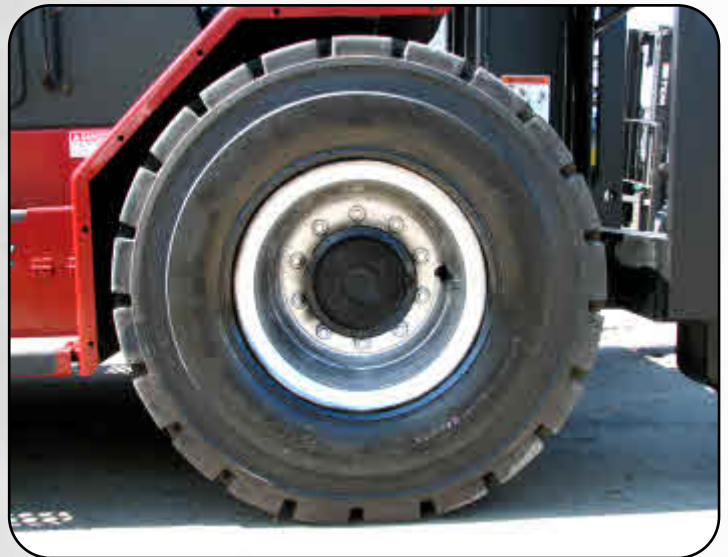
Heavy-duty bolted planetary drive axle
