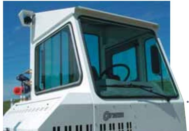
Large glass area and cab design provide excellent visibility to the front, rear and sides.
