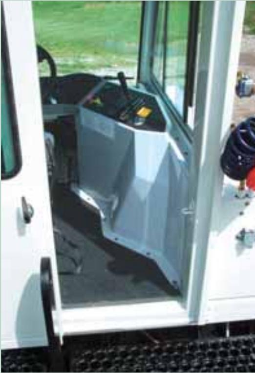
Low, flat floor and wide entryway is designed for no-step entry and exit plus easy sweep-out.
