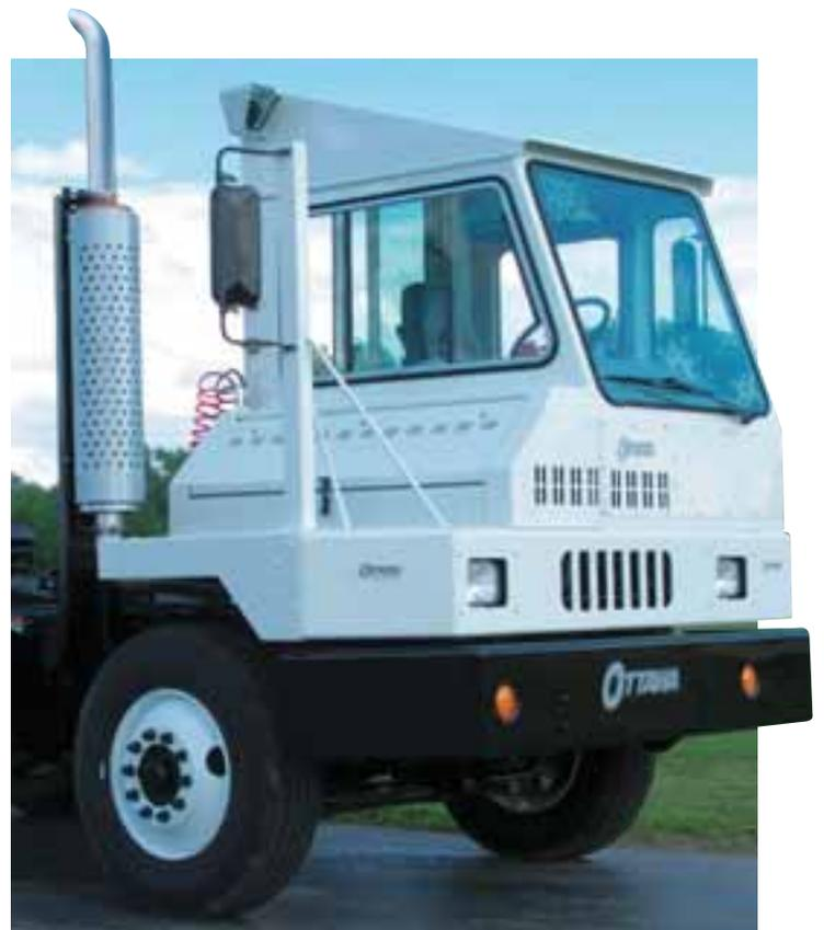
The air-ride cab is designed for quiet comfort, convenience and reduced maintenance. Large cab pivot bushings are designed to help lower cab noise levels and reduce wear to bushings and pins. Raised cab models have no top windows to create solar heating, glare. Electric tilt is standard equipment.
