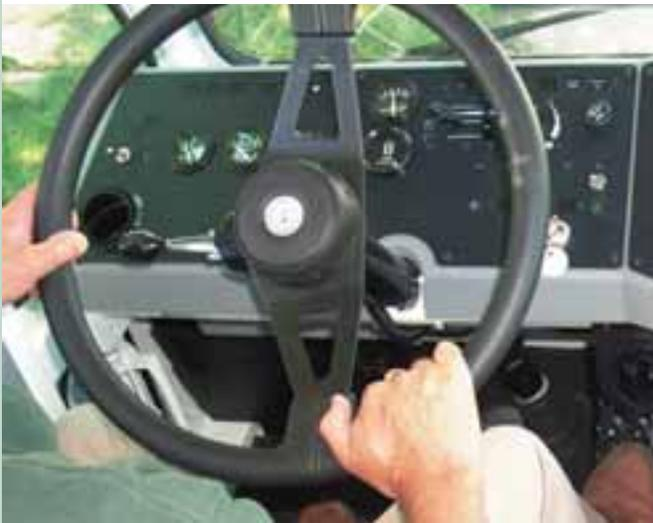
Instrument panel features low-glare, easy to clean ABS material. Heavy-duty gauges are circuit grounded for greater reliability. LED lighting and lighting displays provide long service life. Dash can be serviced without removing steering column.
